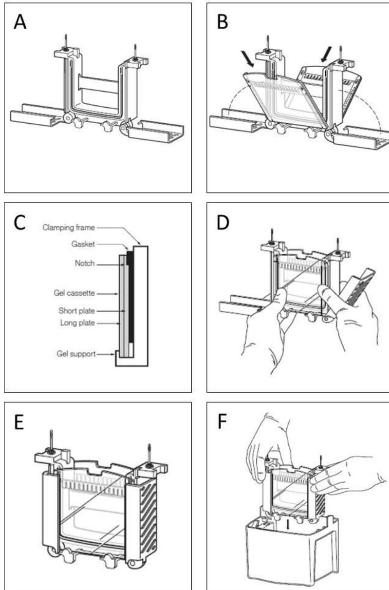
**Figure 12.5 Assembly of Mini-PROTEAN® Tetra Cell for Mini Precast Gels**
