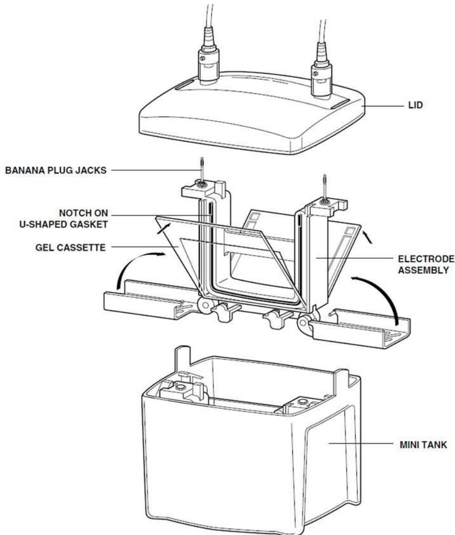
**Figure 12.4 (Assembling the Mini-PROTEAN Tetra Cell (Bio-Rad))**
